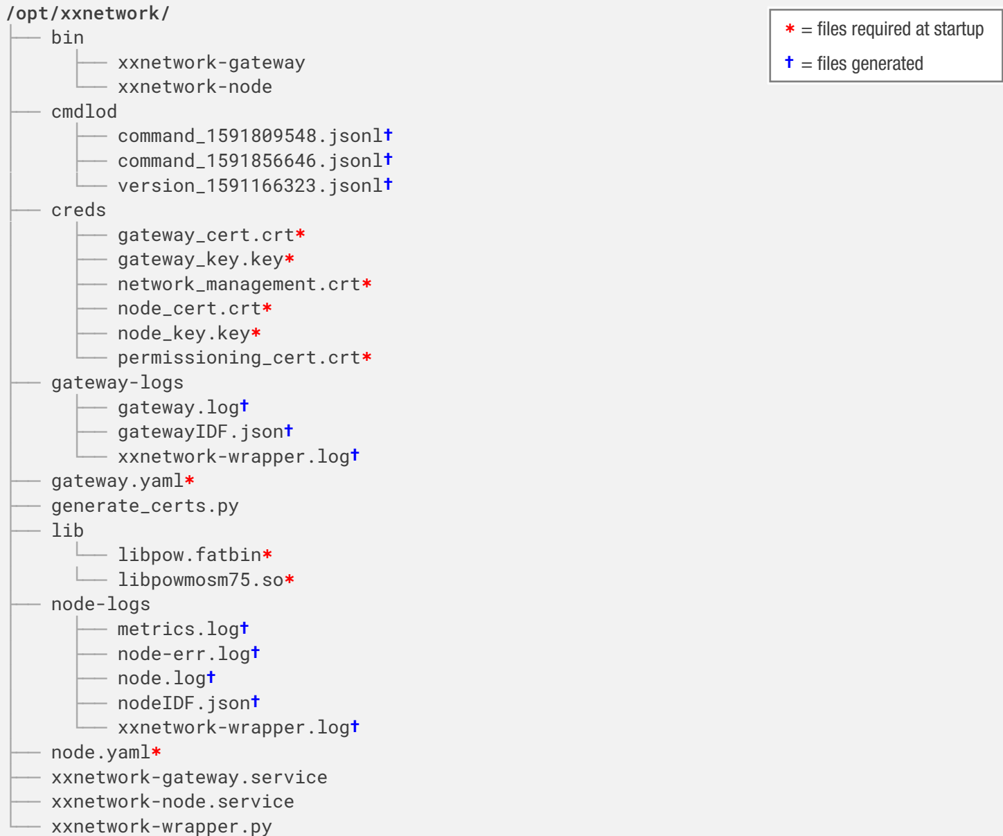
FIGURE 3: Default directory tree when running both Node and Gateway in the default configuration. Files with a red asterisk (*) are required at startup. Files marked with a blue dagger (†) are generated.
